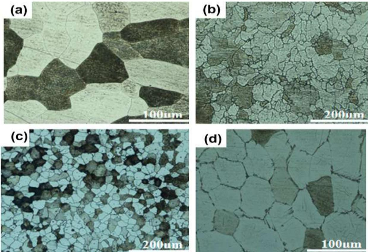
Fig. 3: Microstructure of welds at different grain refinement conditions: (a) aluminium (b) titanium (c) aluminium + titanium (d) cryogenic cooling (Amuda and Mridha, 2012).
