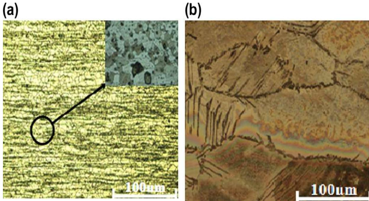
Fig. 4: Microstructure of (a) base metal (b) conventional weld (Amuda and Mridha, 2012).
