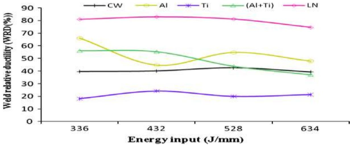
Figure 2: Effect of different grain refinement conditions on weld relative ductility (Amuda and Mridha, 2012).
