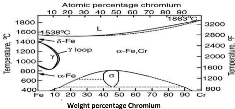
Fig. 1: Fe-Cr phase diagram in FSS (Bhadeshia, *et al.*, 2017)
