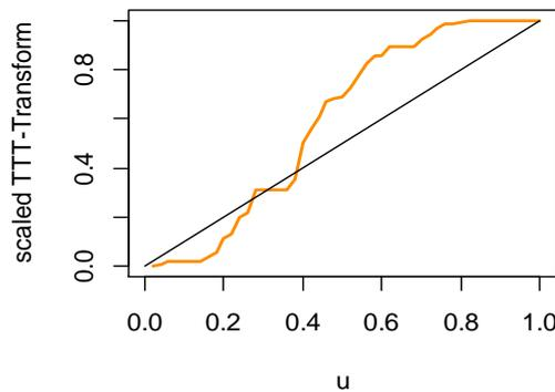
Figure. 6. The empirical scaled TTT-transform plot for Aarset data
