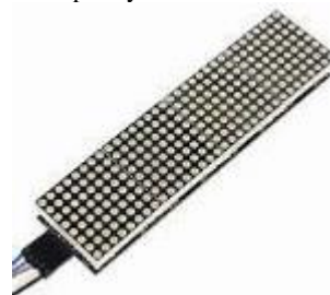
Figure 3: A Multiplexed Dot Matrix Display (Wikipedia, 2023)
