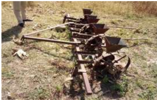
Plate I: Four-row-animal-drawn planter Plate II. Planting process
