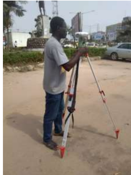
Figure 3: Rover Receiver at One of the Selected Points (RR01) at Ring Road
