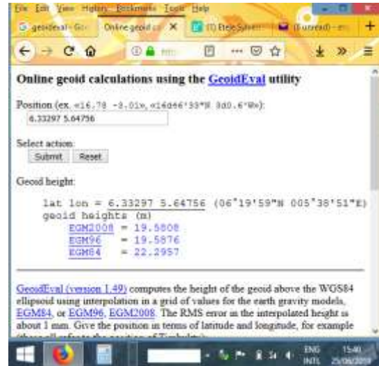
Figure 5: Computation of the Global Geoid Heights of the Points Using GeoidEval Software
