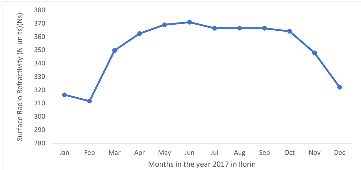
Figure 7: Monthly Variation of Surface Radio Refractivity over Ilorin in the year 2017
