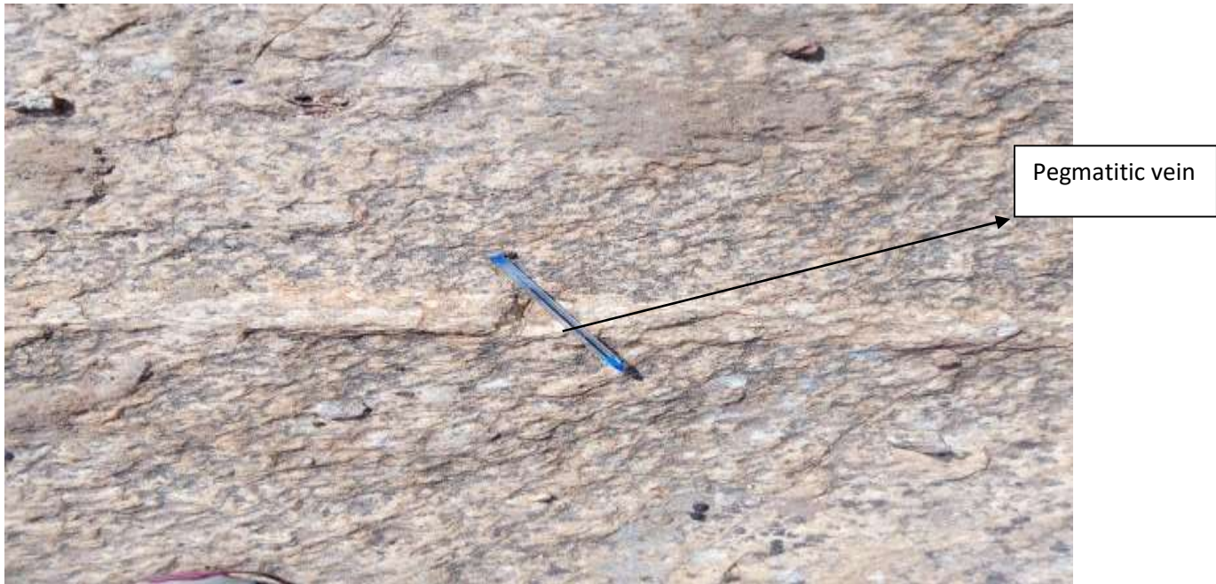
Fig.5: Medium grained granite showing quartz vein intrusion at Tepatan.
