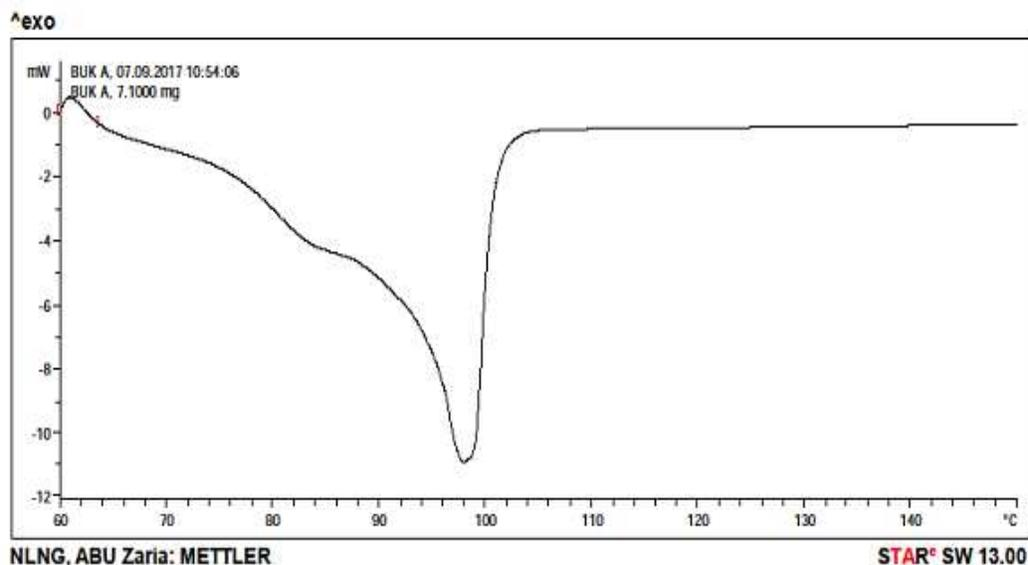
Fig. 1 (a): Thermogram of sample A from DSC experiment
