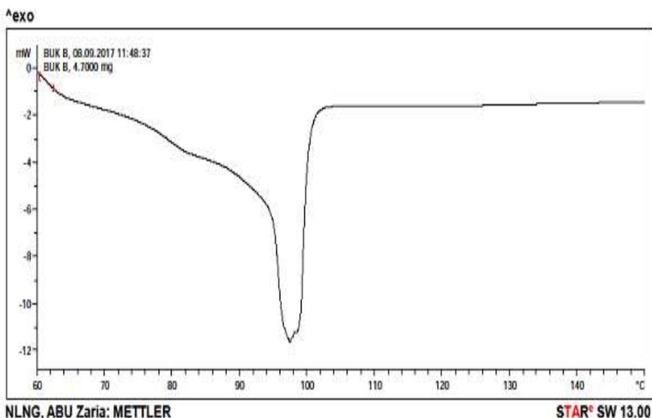
Fig. 1 (c): Thermogram of sample C from DSC experiment
