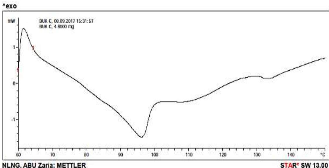
Fig. 1 (b): Thermogram of sample B from DSC experiment
