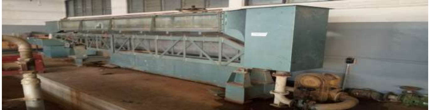
Plate I: side view of the Tilting Flume
