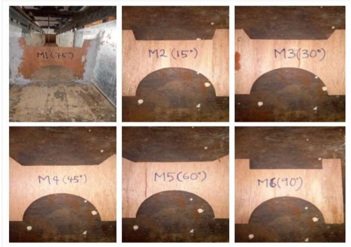
Plate 1: The combined weir-gate models that were fabricated and tested
