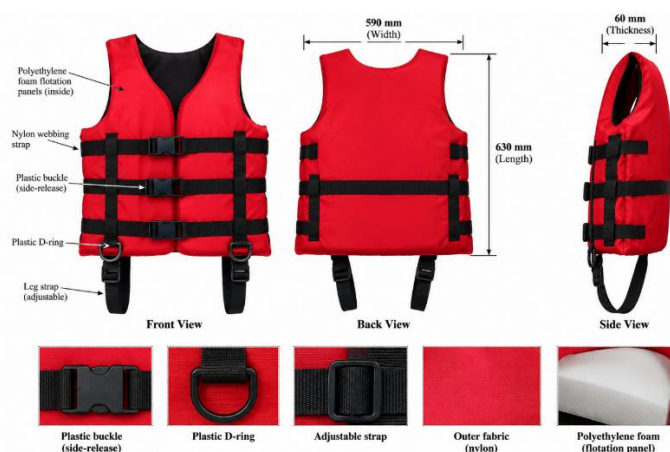
Figure 2: Orthographic Views and Component Identification of the Completed Vest-Type Personal Flotation Device
