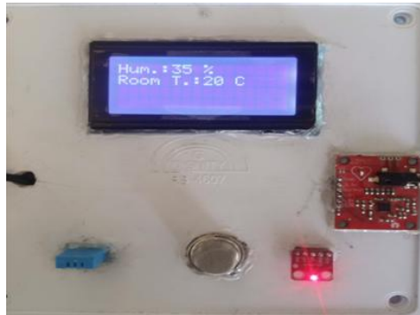
Figure 11: Result Showing Room Humidity and Room Temperature
