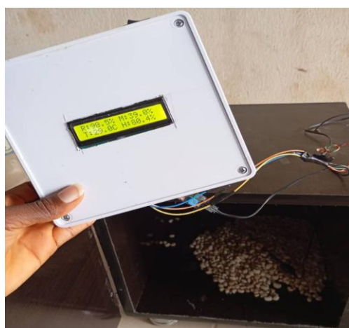
Figure 6: LCD Display Showing Real-Time Risk, Temperature, Humidity, and Moisture Content Values
