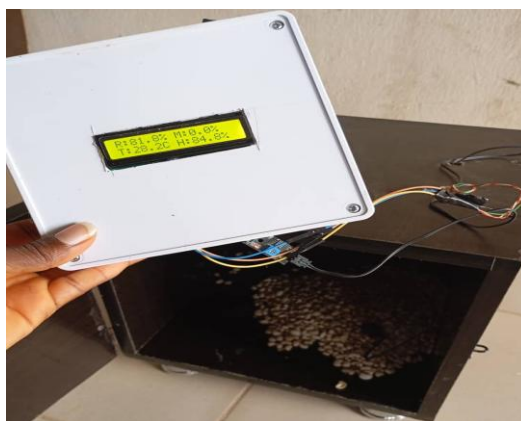
Figure 7: System Display under Safe Storage Conditions
