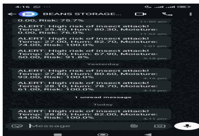
Figure 8: WhatsApp Alert Notification under Critical Storage Condition
