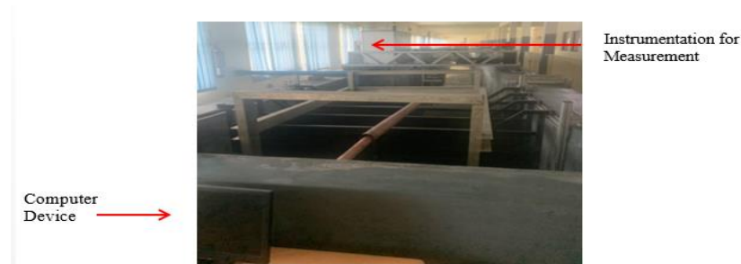
Figure 4: Towing Tank Measurement and Data Collection Device
