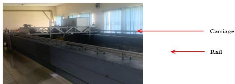
Figure 5: Towing Tank Carriage and Rail.
