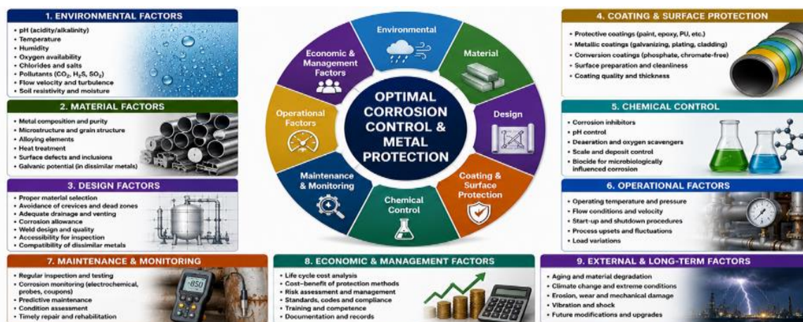
Figure 9: Factors that contribute to corrosion and optimal corrosion control and metal protection techniques (adopted from Melchers, 2020; Kucharlapati et al., 2025; Liu et al., 2026; Manu et al., 2025)
