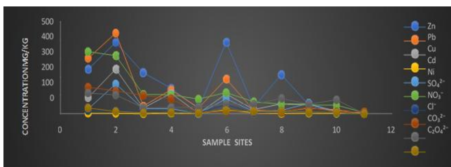
Figure 5: Distribution of Heavy Metals and Ionic Species at the Study Sites (mg/kg)
