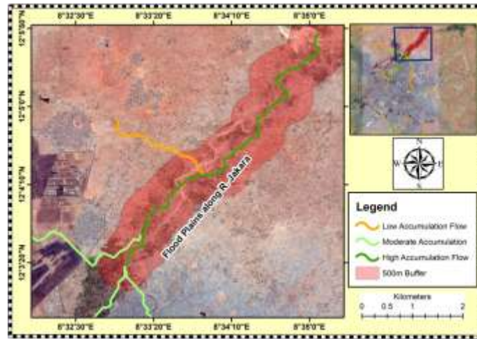
Figure 11: High Surface Accumulation Flow Area showing part of Residential Landuse along the Floodplains of River Jakara at High Flood Risk level within 500m Distance
