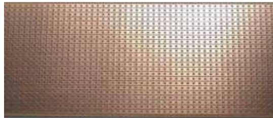
Fig. 8: diagram of a Vero-board
