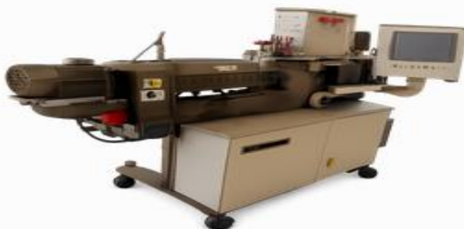
Figure 1: Berker Perkins MPF twin-screw extruder with co-rotating and intermeshing screws
