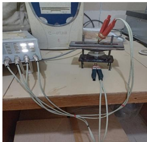
Plate 5: The Setup LCR Machine with a Sample
