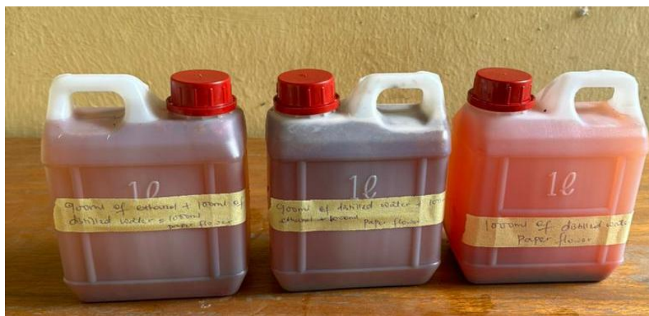
Figure 2: Dye Extracts from B. glabra Bracts Using 90 % Ethanol (A), 10 % Ethanol (B) and Aqueous (C)
