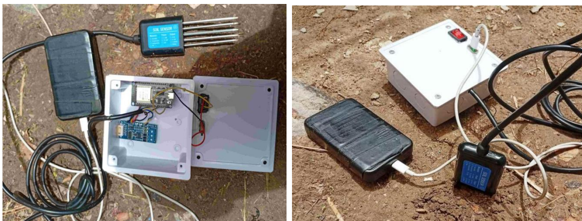
Figure 3: Field Deployment of the CWT-Soil-THC-5 Sensor
