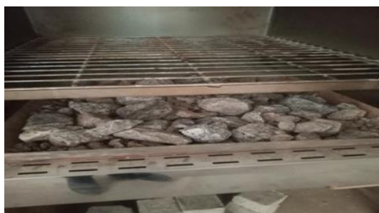
Figure 1a: Clean Ballast Dried in an Oven for 24 Hours
