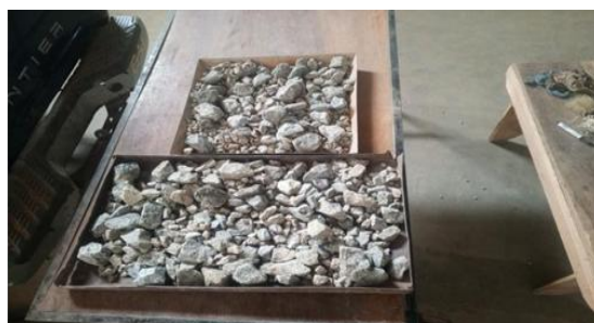
Figure 1b: Ambient temp cooling of clean ballast
