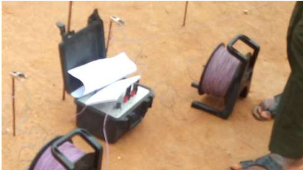
Plate 2. Terrameter, wire cables and reels
