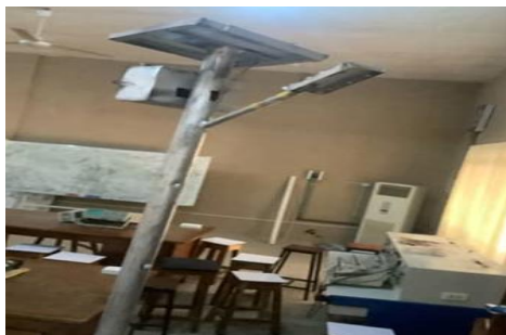
Figure 12: Prototype of the Automatic Solar Power Streetlight System
