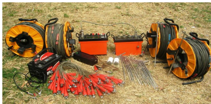
Figure 2: Abem Terrameter SAS 1000 used for the Data Acquisition showing the 4 Electrodes, the Cable Rollers and the Terrameter Box Device
