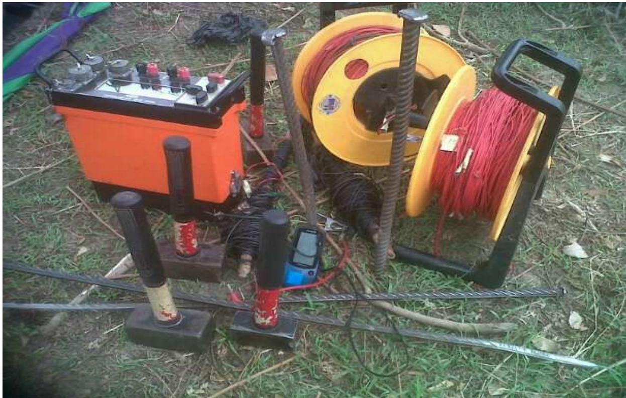
Fig. 5: ABEM Terrameter (SAS 1000) and other equipment to carry out the research.
