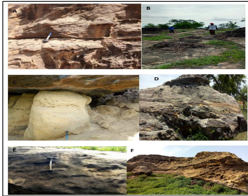
Plate I: (a) Planar Cross Bed (b) Strike Slip Fault (c) Small Trough Cross Bed with fine Grained Ripple Cross Lamination and Erosional Surfaces (d) Load Cast (e) Small Scale Trough-cross Bed (f) Highly Bioturbated Bima Sandstone with Planar Cross Bed
