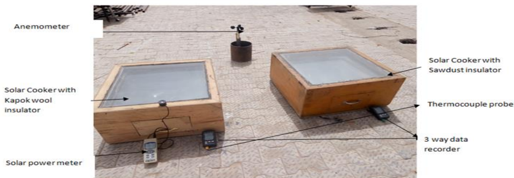
Plate 2: Experimental Set Up of the Two Similar Solar Box Cookers
