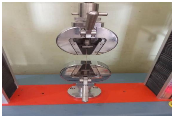
Plate. I. Determination of the Tensile Strength of the Doum Palm Fibre
