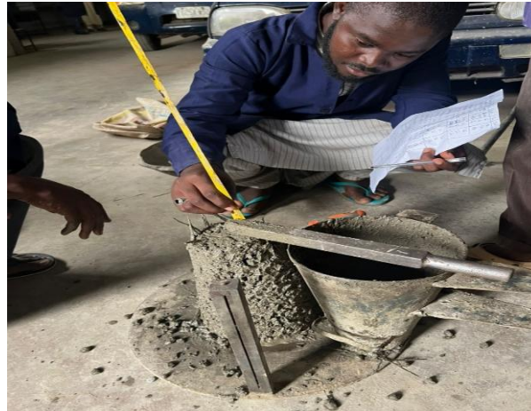
Plate II. Determination of Slump Value for the Fresh Concrete
