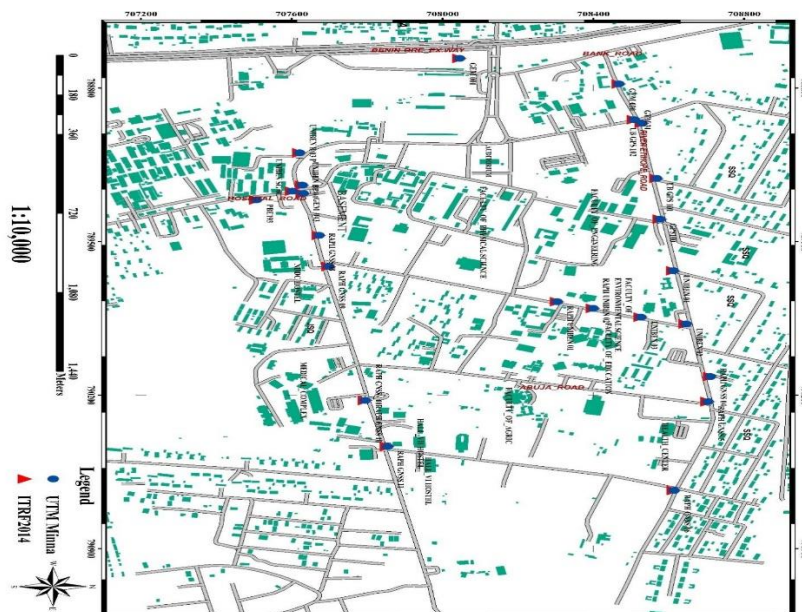
Figure 9: Plot of controls overlay in UTM-Minna and ITRF2014
