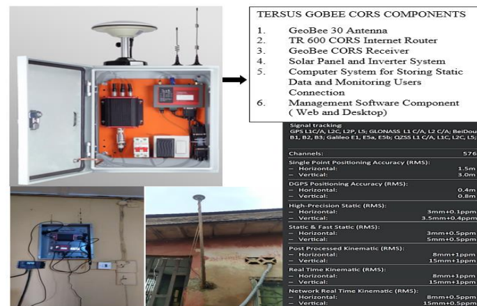
Figure 2: The CORS_Geosystems Parameters and Location (Ehigiator-Irughe and Oladosu 2023)
