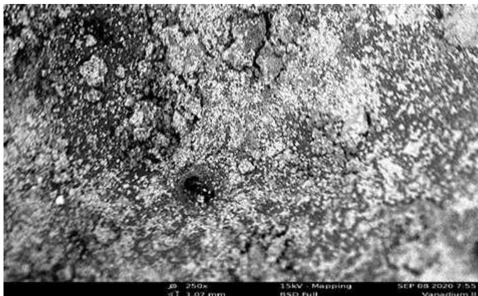
Figure 3: SEM image of Vanadium (III) salts plus ligands SEM IMAGES AFTER GRINDING
