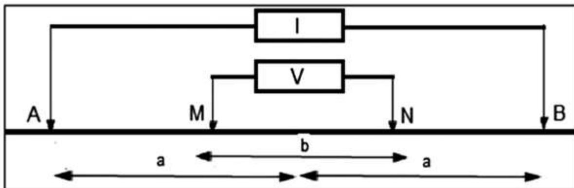
Figure 2: Electrode arrangement in the field - VES Schlumberger electrode array (yusuf et al., 2018)
