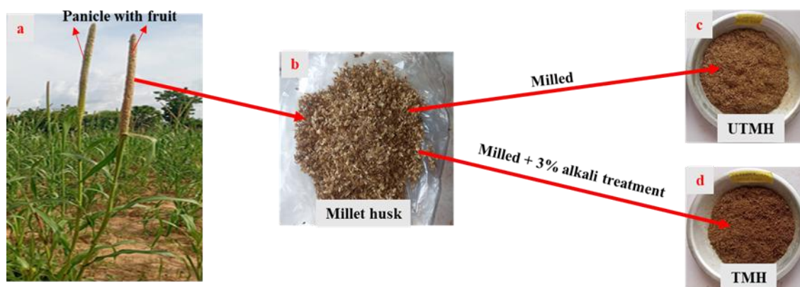
Figure 1: Millet husk preparation from (a) panicle with fruit, (b) millet husk, (c) UTMH, and (d) TMH
