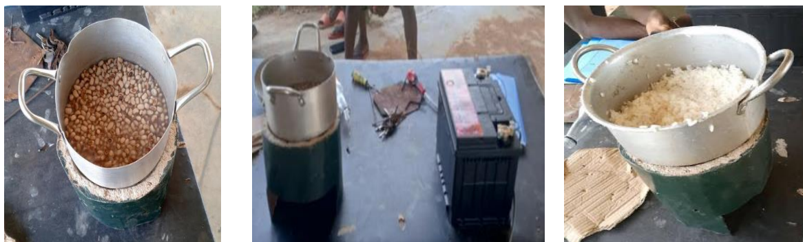
Figure 4(a-c): WBT and CCT showing setup and products, (a) Cook beans (b) Boiling water (c) cook rice
