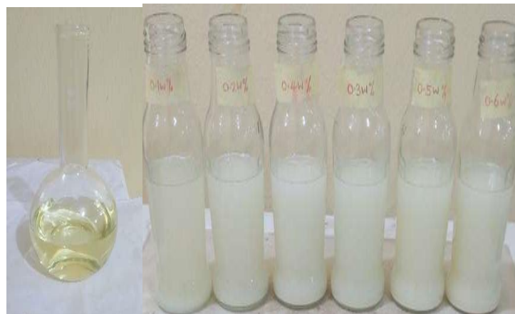
Figure 1: Prepared ME and Nanofluids with Eight-Times Coated TiO 2 Nanoparticles
