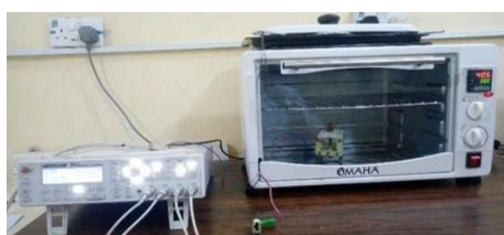
Figure 4: Relative Permittivity and Loss Measurement set - at Different Temperatures
