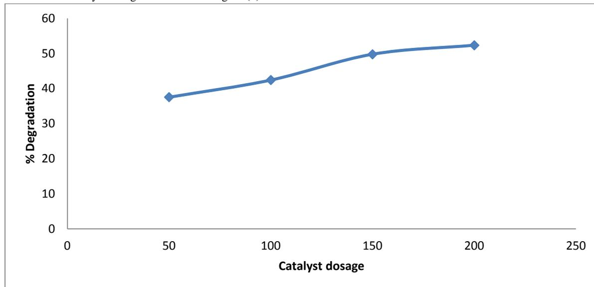
Fig. 5: Effect of catalyst dosage on degradation of MR using Cd-Al/C LDH.
