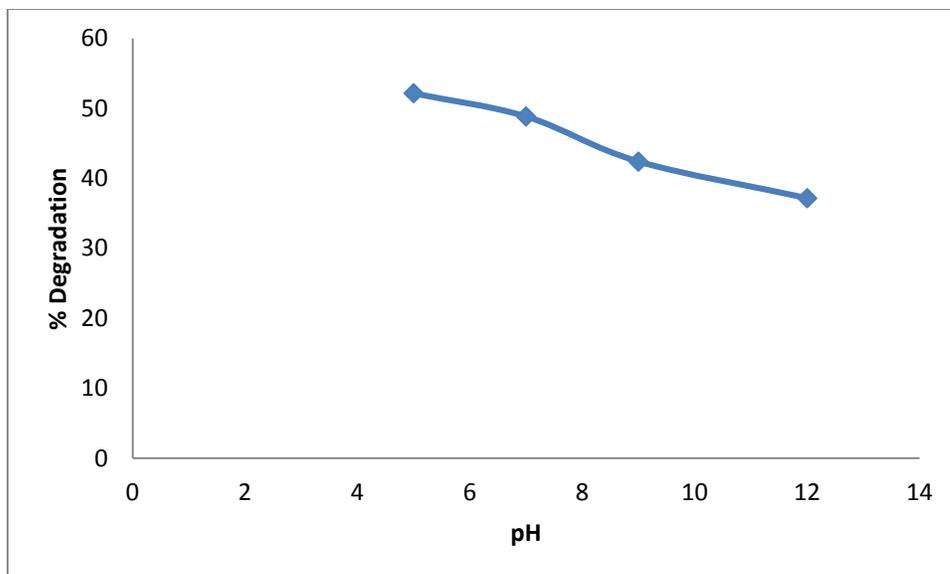
Fig. 6: Effect of pH on degradation of MR using Cd-Al/C LDH.
