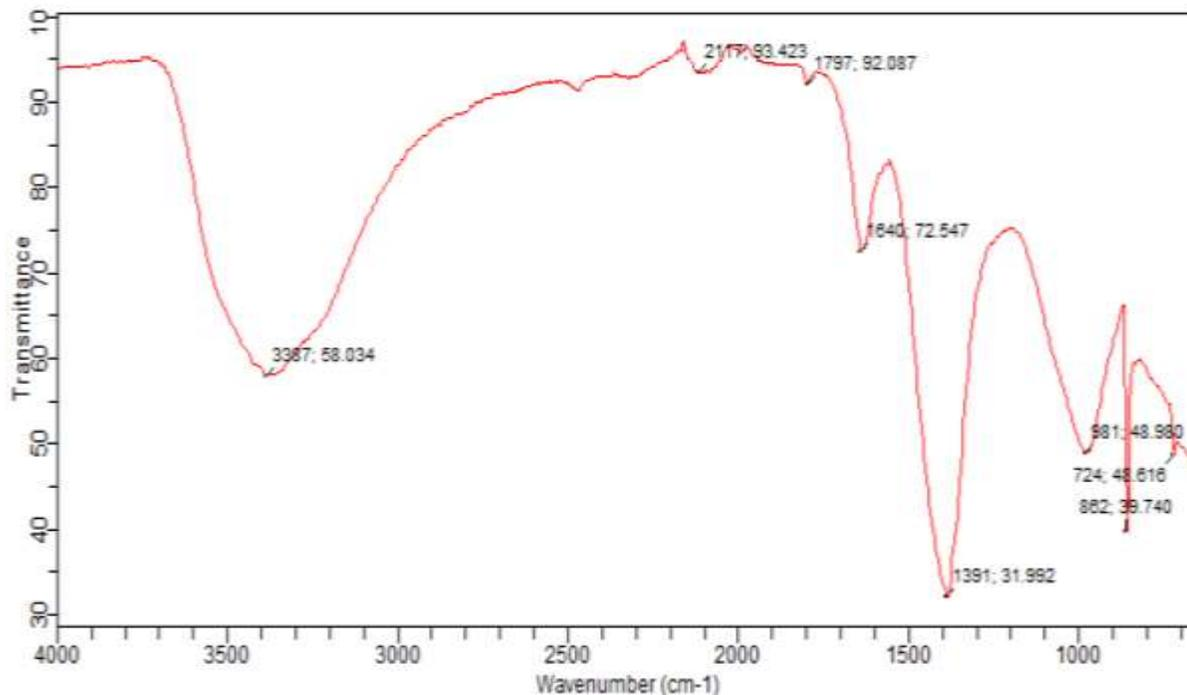
Fig. 3: FT-IR Spectra of Cd-Al/C LDH
