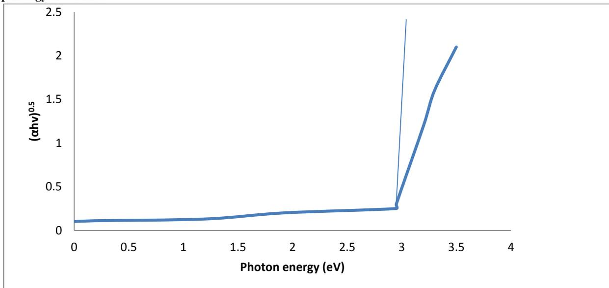
Fig. 4: The Tauc plot showing the energy band gap of Cd-Al/C
