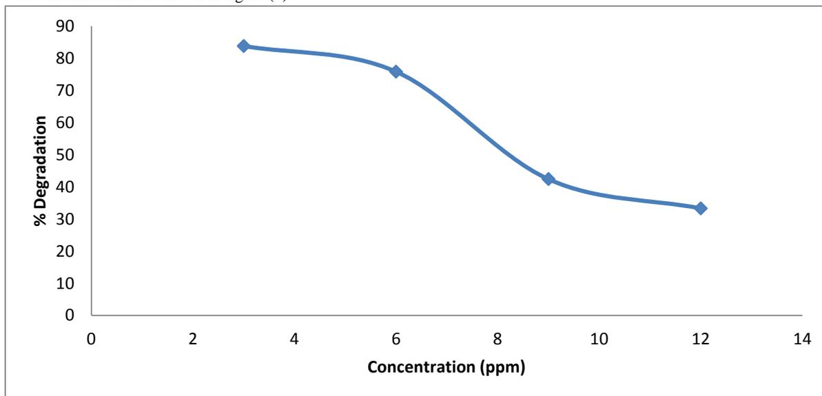
Fig. 7: Effect of concentration on degradation of M.R using Cd-Al/C LDH.
