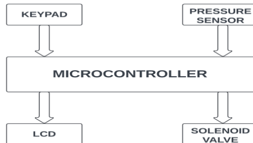
Figure 2: Inflation Monitor Block Diagram
