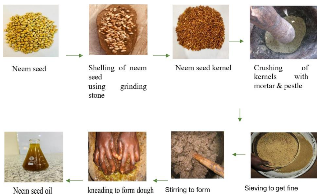
Figure 1: Procedures of traditional extraction of neem seed oil
