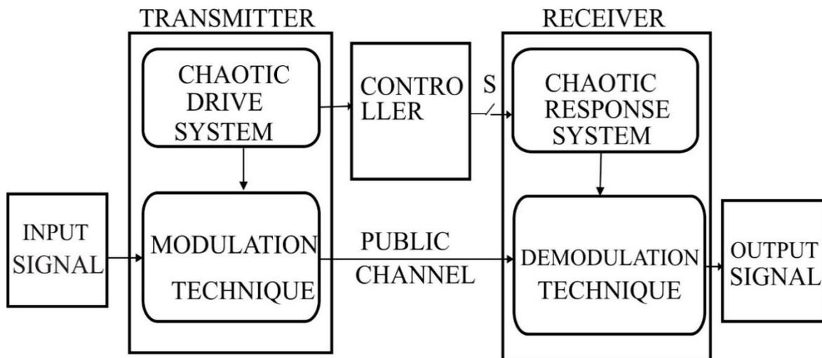
Figure 3: Block diagram of the chaotic communication system
