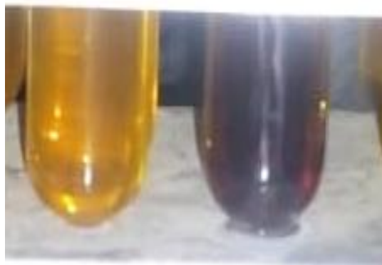
Figure 1: DNS assay tubes showing color development due to the release of reducing sugars from CMC hydrolysis by fungal cellulase
