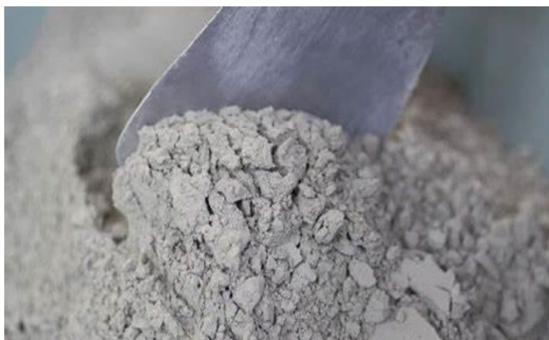
Figure 3: Portland cement fine powder (Desharnais, 2019)
