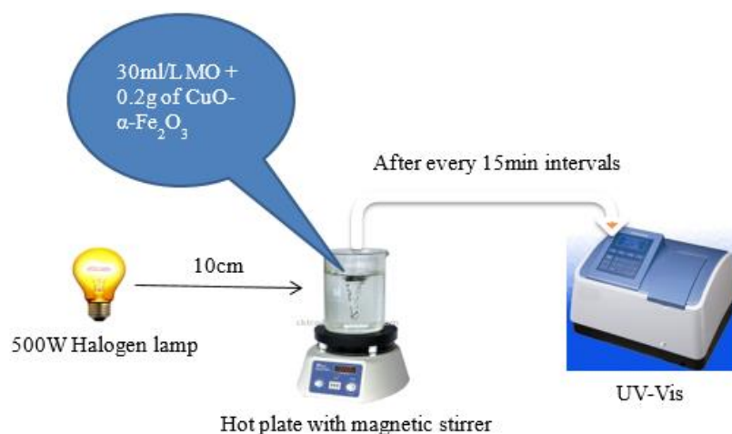
Figure 3: Experimental set up for the Photocatalytic degradation of MO dye
