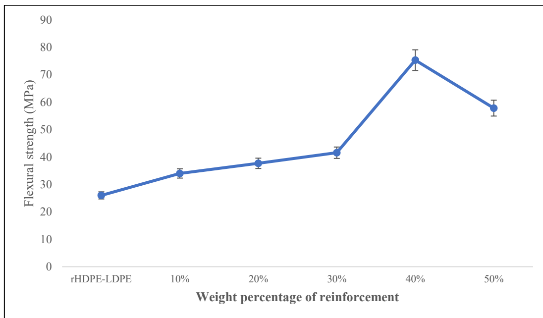
Figure 5: Effect of BAP on the flexural strength of recycled HDPE-LDPE blends
