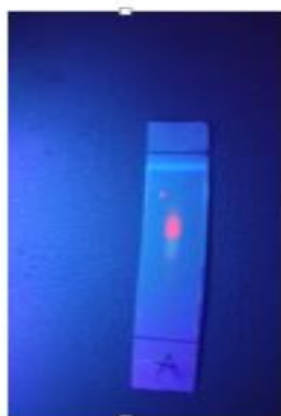
Figure 11: The T.L.C profile of n-hexane under UV lamp
