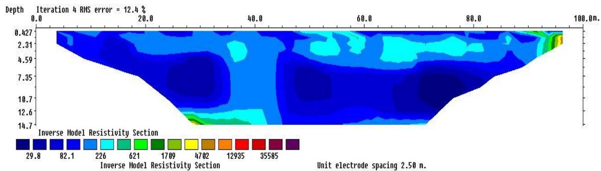
Figure 10: Results of 2D electrical inversion of Dipole-Dipole array along profile 6
