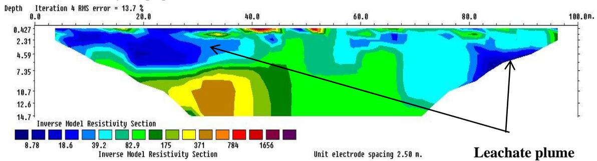
Figure 5: Results of 2D electrical inversion of Dipole-Dipole array along profile 1
