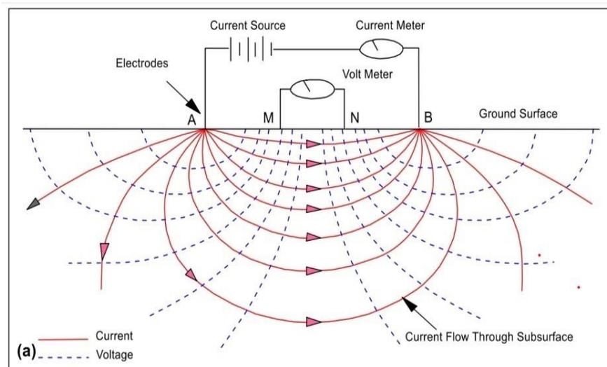
Figure 3: Fundamental conceptual model for resistivity measurement (modified after Todd and Mays 2005)
