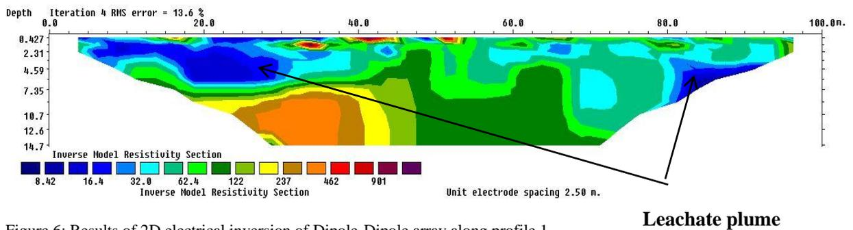
Figure 6: Results of 2D electrical inversion of Dipole-Dipole array along profile 1
