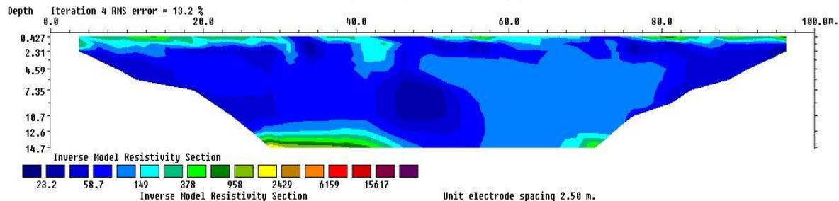
Figure 12: Results of 2D electrical inversion of Dipole-Dipole array along profile 8
