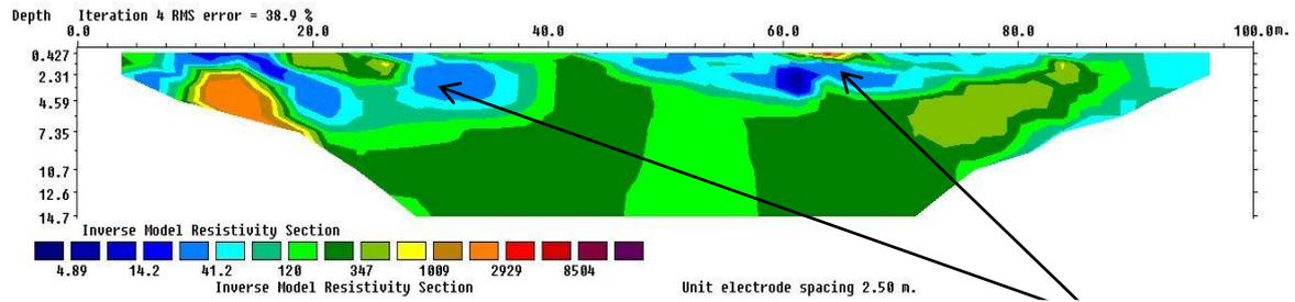
Figure 8: Results of 2D electrical inversion of Dipole-Dipole array along profile 4
