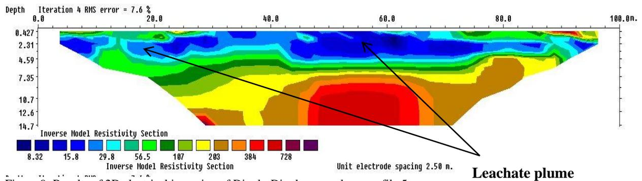
Figure 9: Results of 2D electrical inversion of Dipole-Dipole array along profile 5
