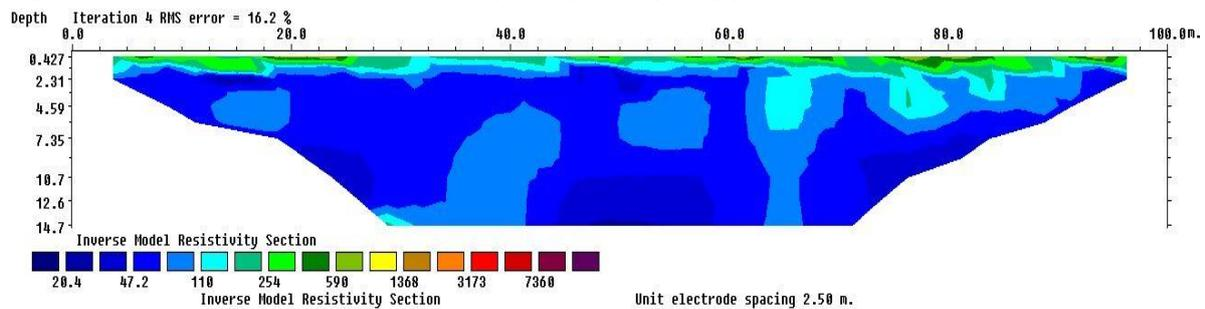
Figure 11: Results of 2D electrical inversion of Dipole-Dipole array along profile 7
