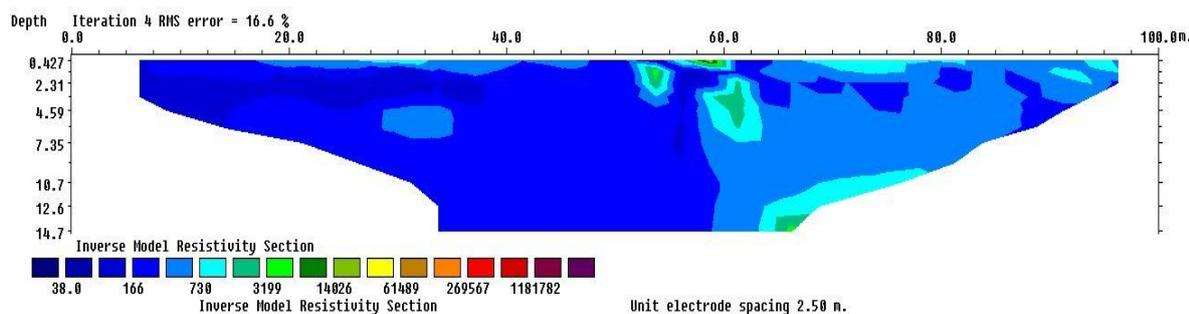
Figure 13: Results of 2D electrical inversion of Dipole-Dipole array along profile 9
