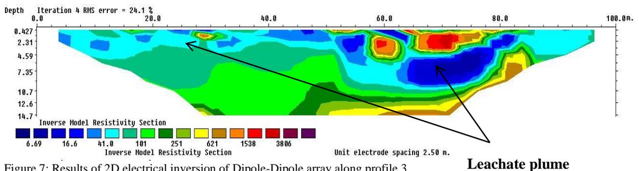
Figure 7: Results of 2D electrical inversion of Dipole-Dipole array along profile 3
