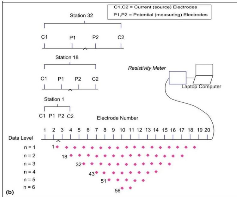
Figure 4: Principle diagram to generate a pseudo section in ERI
