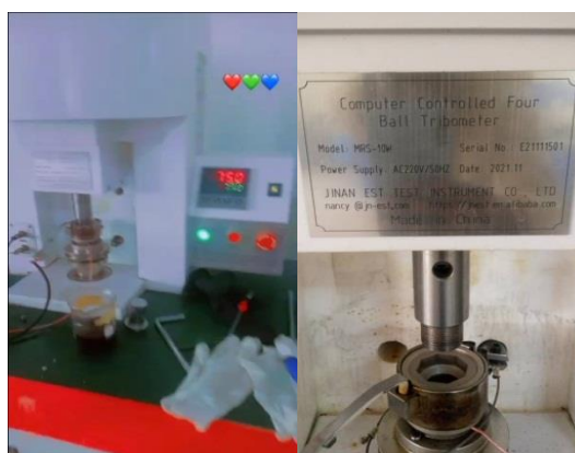
Plate 2: Experimental set up for tribological analysis
