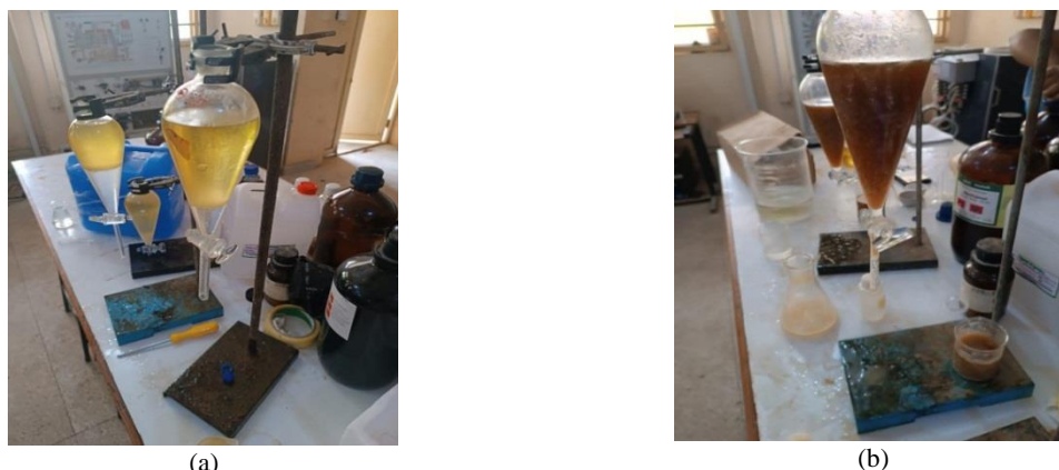
Plate 1: Esterification of Palm kernel oil and castor oil (a) Palm kernel oil (b) Castor oil
