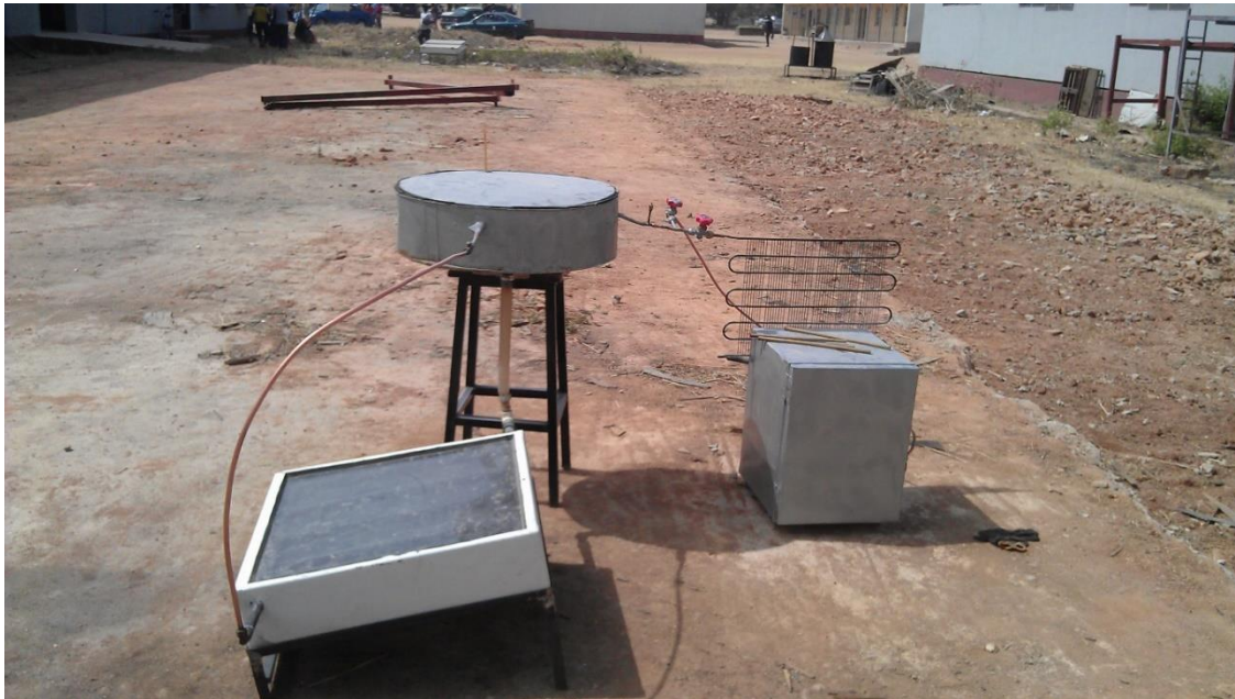
Plate 1: The system assembly of the solar adsorption refrigerator
