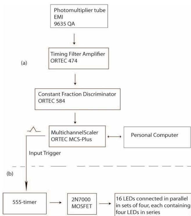
Figure 1: Schematic diagram of the pulsing system showing the arrangement for detecting and recording time-resolved optical luminescence spectra (a) and the pulsing circuitry used to pulse the light emitting-diodes (b)
