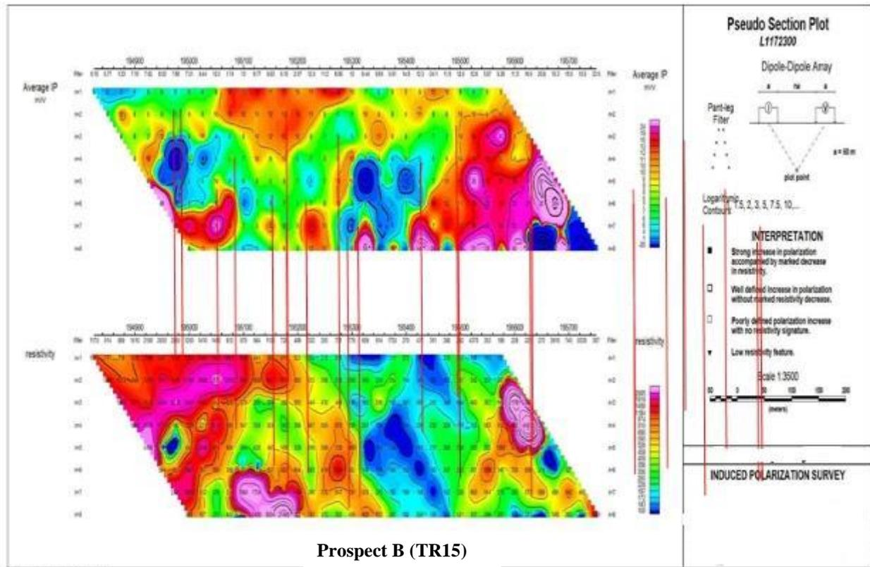
Figure 6: Pseudo-section plot of the IP and resistivity data for Prospect B
