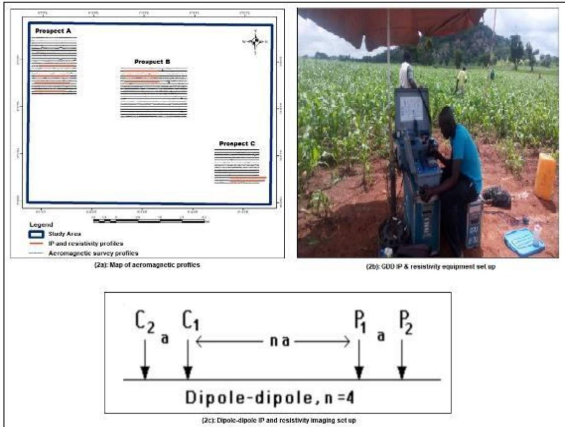
Figure 3: Geophysical data acquisition methods
