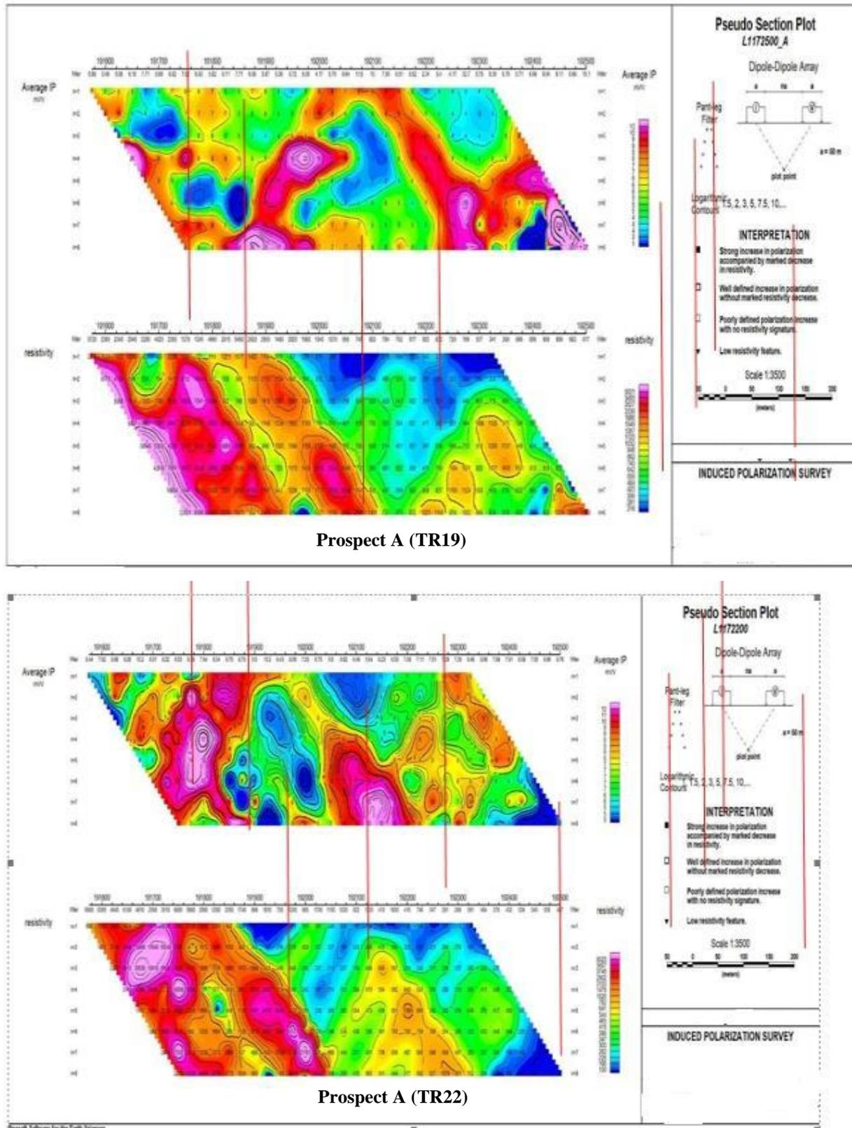
Figure 5: Pseudo-section plot of the IP and resistivity data for Prospect A
